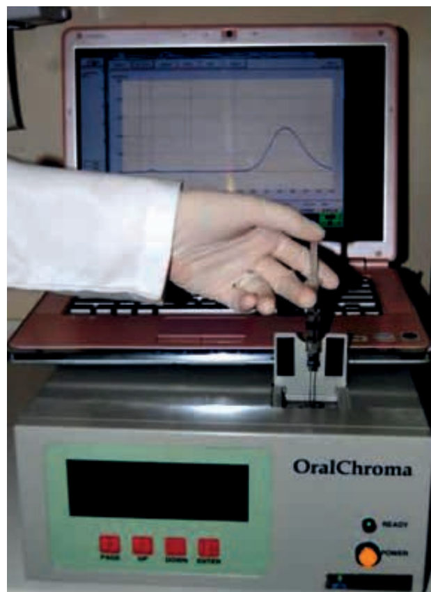
Fig. 3. The Oral Chroma™ device connected to a computer during injection of a sample.
